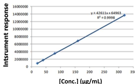
**Fig. 3.** Calibration curve used for Galantamine quantification extracted from *L. aestivum*.
